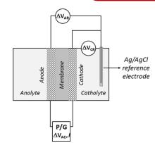
The aqueous phase in our study allows the utilization of a standard Ag/AgCl reference electrode for monitoring the anodic and cathodic overpotentials.
