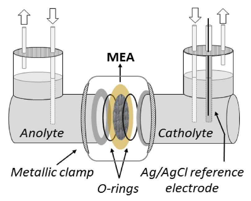
A standard Ag/AgCl reference electrode allows for monitoring the anodic and cathodic overpotentials. Ohmic overpotential was quantified via Electrochemical Impedance Spectroscopy.
